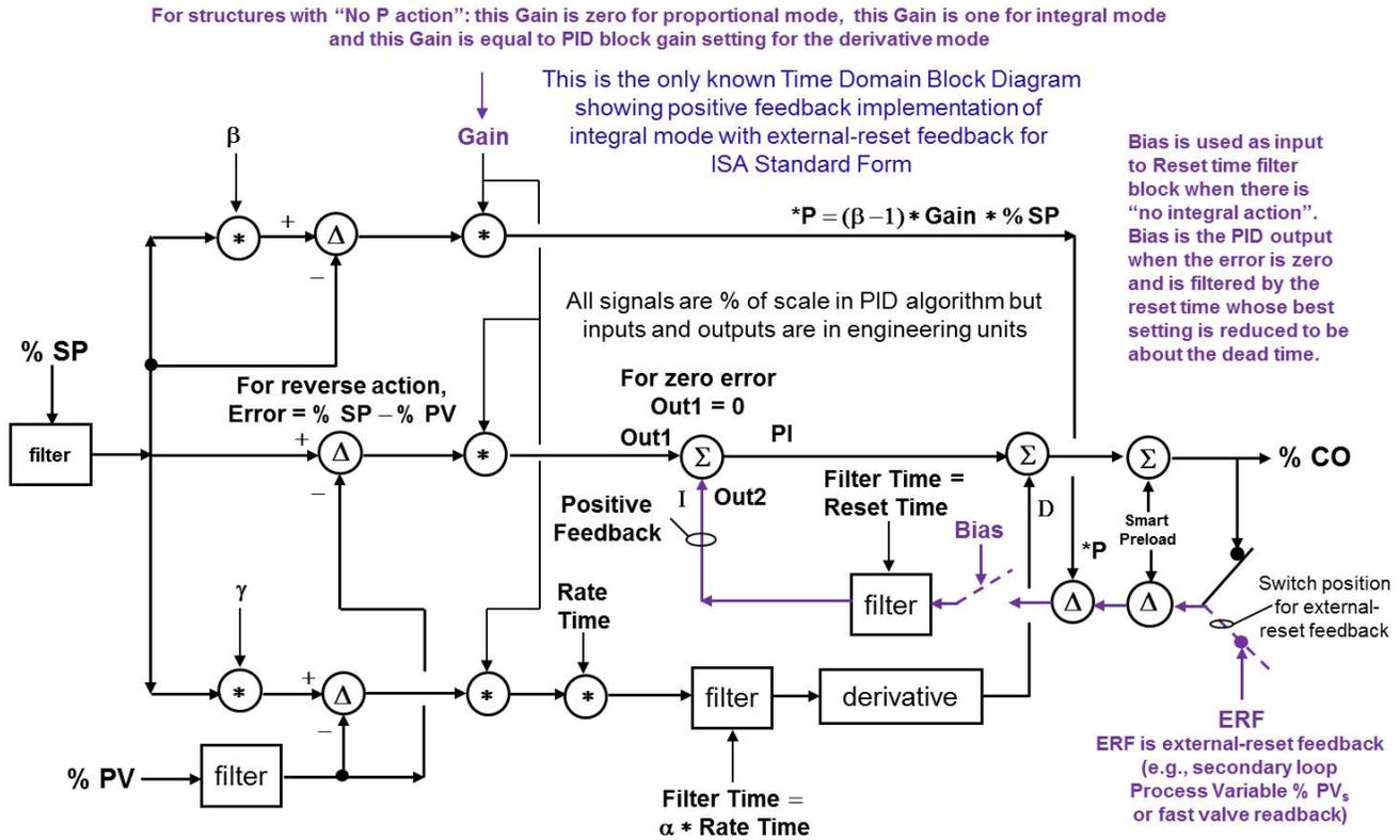
Figure 1 Positive feedback implementation of integral action for standard form PID
