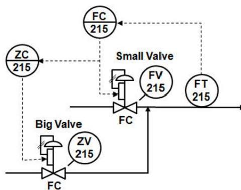
Figure 5 Valve position control increases precision and rangeability <sup>13</sup>
