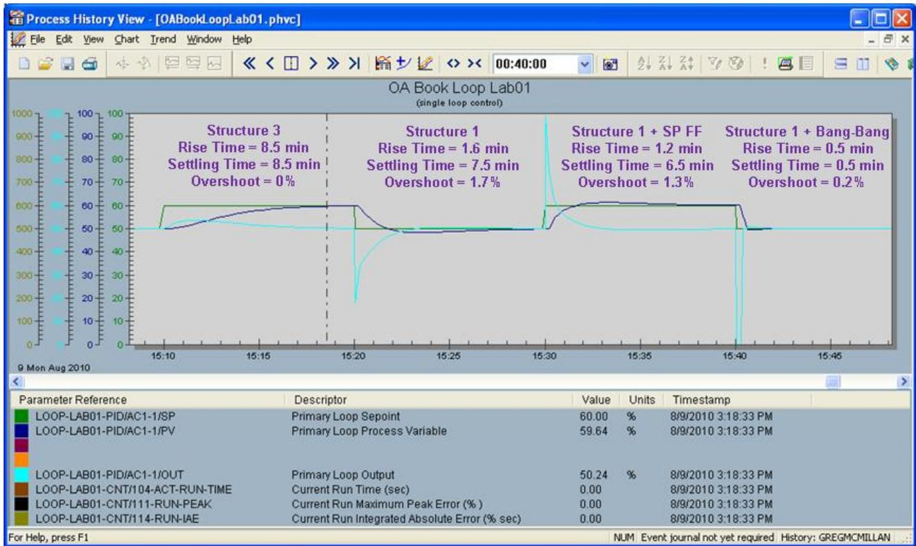
Figure 2 Effects of structure, setpoint feedforward, and Bang-Bang logic on setpoint change for an integrating process
