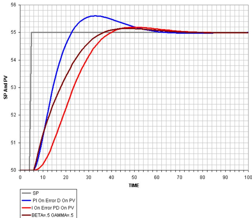
Figure 4 Self-regulating process response to a setpoint change for three different structures<sup>14</sup>.
