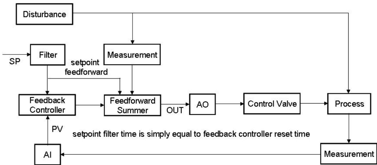
Figure 3 Configuring a SP filter in the feedback controller prevents overshoot and adding SP feedforward reduces rise time<sup>11</sup>.
