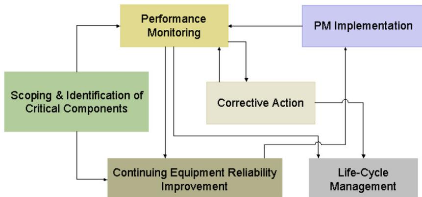
Figure 1- INPO AP-913 Equipment Reliability Process
